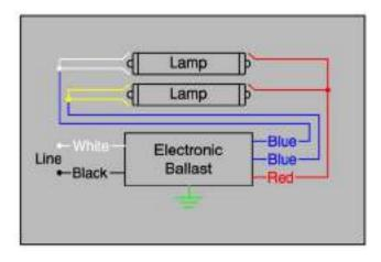
Notes: Applicable for 120V and 277V magnetic T12 to either T8 or T12 electronic fixtures. Always disconnect power to lighting fixture prior to servicing the fixture.
